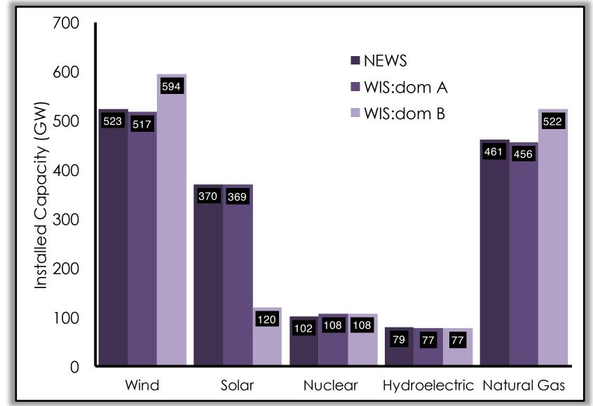
As "cost" parity is approached the installed capacities tend to: wind = solar PV = natural gas
